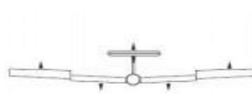
Like FLAPERON and AILEVATOR, AIRBRAKE is one function that is really made up of a series of pre-programmed mixes all done for you within the radio. AIRBRAKE (often called "crow" or BUTTERFLY - see GLID, p. 62 for details) simultaneously moves the flap (if installed), twin ailerons (if installed) and elevator, and is usually used to make steep descents or to limit increases in airspeed in dives.
