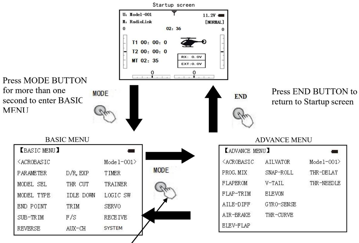
Press MODE BUTTON to switch between BASIC and ADVANCE MENU
