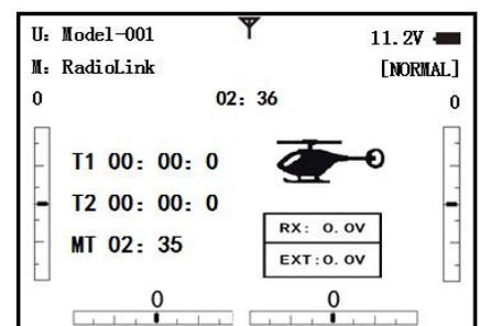
Find telemetry information: under BASIC MENU, select RECEIVE, presses PUSH to enter, you can find the telemetry info, shown as below. RX is receiver voltage, EXT is external voltage. Also temperature and engine speed (EXT, TEMPERATURE, RPM, and GPS all need telemetry sensor).
