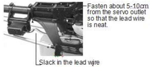
• After the servos are installed, operate each servo over its full travel and check that the pushrods and servo arms don't bind or contact each other. Also make sure the controls do not require excess force to operate. If there is an objectionable buzzing sound coming from a servo, there is probably too much resistance in the control. Find and correct the problem. Even if there is no servo damage, excess battery drain will result.
