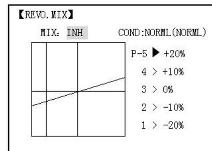
Note: The throttle and pitch curves for the normal condition is always on. They cannot be inhibited. The other four conditions are activated with their throttle curves or throttle hold.
